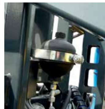
**Quadrilever** pantograph lifting system of the boom with parallelogram by 2 hydraulic cylinders. It is all aided by a hydro-pneumatic system with nitrogen bowls. The joints of the lifting device are realised with self-lubricating pins and adjusted steel pins. The Quadrilever system assures great stability for the boom, both during treatment and during transfer, also allowing greater extension in height compared to classic vertical lifting mast.
