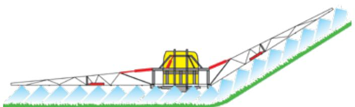
**BL-System:** automatic ground contour boom alignment system, by means of the boom hydraulic equalizer and sonars. Also, it is possible to automatically lift the boom at field ends, and its return to the established height once steering is completed.
