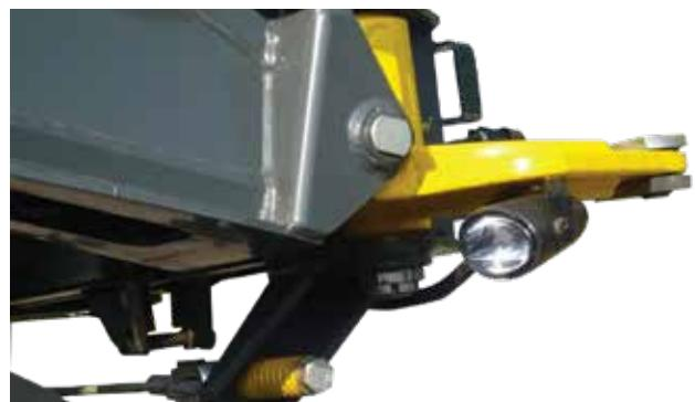
**Set LED night-work lights:** positioned in the centre of the bar, these special long beam lights enable visibility of the nozzles during night-time treatments.
