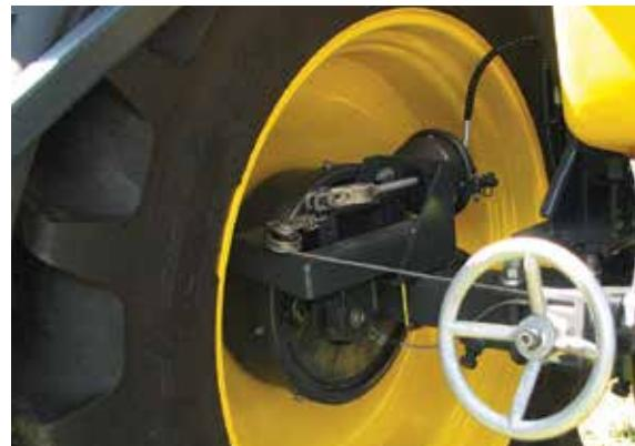
Brakes: these are available in hydraulic or pneumatic, with manual control or automatic with the tractor pedal. Road regulations of 25km/h or 40 km/h or 50 km/h (Germany).
