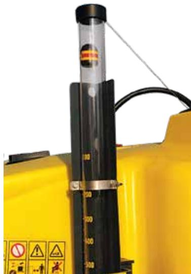
The dry-type level gauge is visible from the tractor and from the filling side, for an easy read of the liquid quantity inside the tank. The feeder, which is positioned in the middle of the tank, is less affected by sprayer chassis uneven standing.
