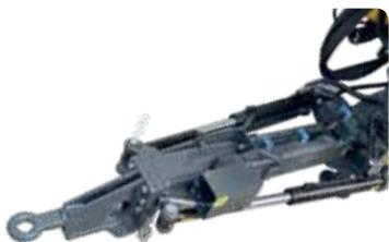
Hydraulically activated steering drawbar. Compatible for Trailmatic & Trailmatic Profi electronics management.
