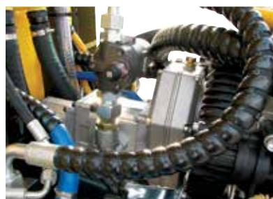
The fan can be actioned directly by the hydraulic pump of the tractor or by an independent system (look at the picture) actioned by the cardan shaft together with the pump of the sprayer. The system is consisting of: hydraulic pump, oil tank with filter and outside level gauge.
