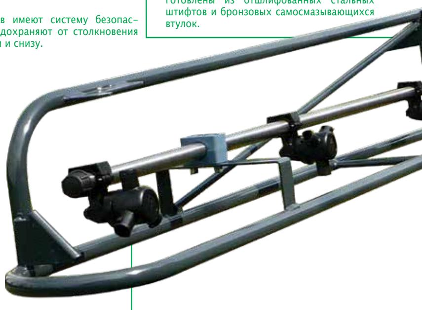
The nozzles and tips are protected inside the boom structure in order to avoid any contact with the ground or obstacles. The pipes are in stainless steel. The trijet nozzles are fitted with anti-dripping membrane device, shutdown position and the ring nuts are of the quick coupling type.
