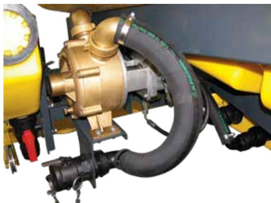
**Centrifugal pump:** these are available as optional for loading activated by hydraulic motor with flow rates of 250 and 500 l/min.
